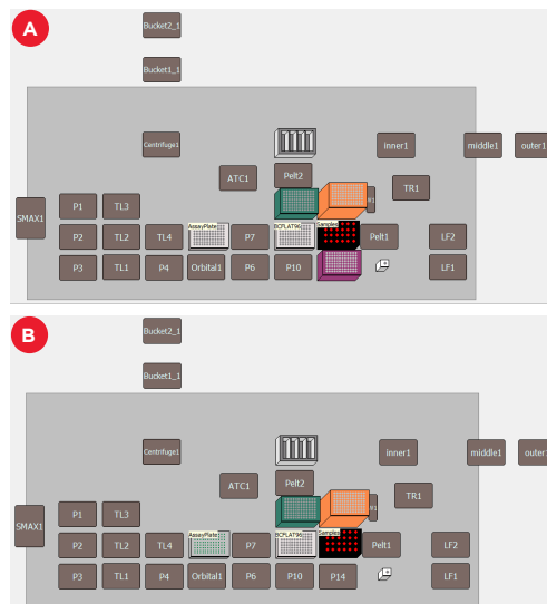
Figure 3. Biomek i7 Hybrid Deck Layouts. Deck layouts of automated ThermoFisher Easy-Titer (A) and ValitaCell ValitaTiter (B) IgG quantification assays. Together the automated method required the following deck components: 7 1X1 ALPs, Orbital Shaking ALP, and an integrated Molecular Devices SpectraMax i3x.
